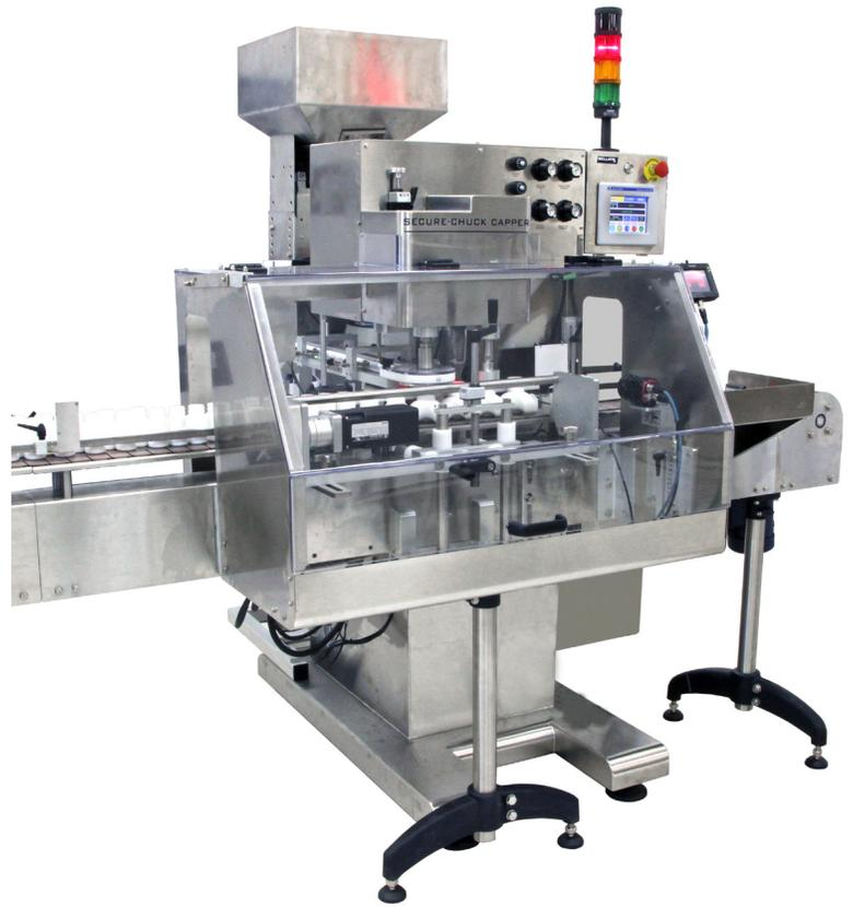
*This photo shows a secure chuck capper. Photo provided by BellatRX*
